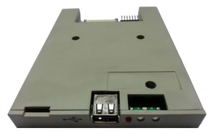
\* Need to format usb flash with floppy to usb software before working on this type of floppy drive to emulator
