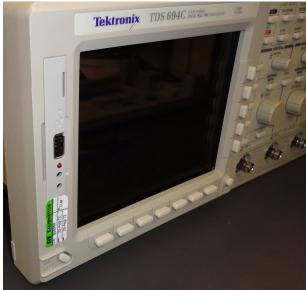
The gap betwee n the emulato r and the wider Tektron ix bezel opening can be covered with with a small
