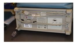
Remove 4 screws from rear bezel (T20 driver)
