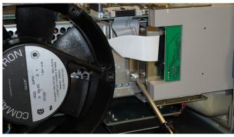
Remove 2 screws from floppy mounting bracket (T15 driver). Slide
