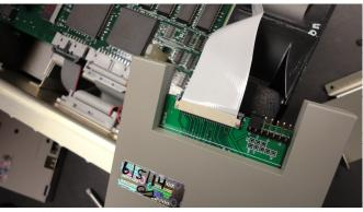
Insert flex tail into emulator connector as far as possible and using a flat tool, gently press the
