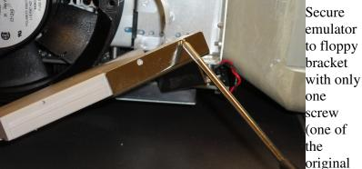
floppy screws fits better than the new screws supplied with the emulator in this instance). The floppy drive was wider than the emulator as it had allowance for an end located floppy eject button on some models. The emulator will be secured by the single screw and the front bezel of the scope.
