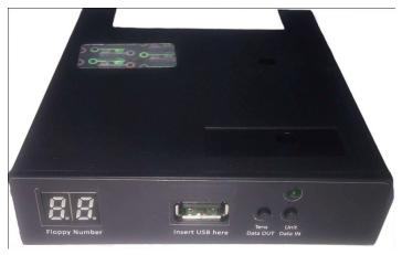
3) With the help of switches provided in front of emulator, change to block on which you copied the data on computer. You can just starting reading of writing the necessary files directly from the usb disk. In this version of floppy drive to usb emulator any changes are directly done on the flash drive. The green indicator will be on while reading and writing.
