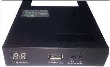
(means that the first 1.44 mb data is the selected folder is being copied into the internal memory of usb as floppy drive emulator).
