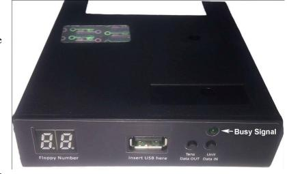
you will see that the display has changed from 00 to D0 (means that the first 1.44 mb data is the selected folder is being copied into the internal memory of usb as floppy drive emulator).
