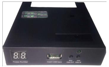
3) With the help of switches provided in front of emulator, change to block on which you copied the data on computer. You can just starting reading of writing the necessary files directly from the usb disk. In this version of floppy drive to usb emulator any changes are directly done on the flash drive. The green indicator will be on while reading and writing.
